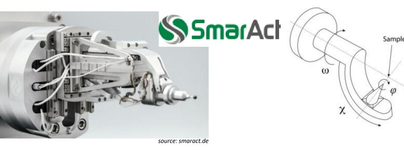
Initially developed based upon PSI's 6-axis-goniometer for protein crystallography PRIGo, SmarAct GmbH's SmarGon is a now commercially available positioning device allowing 4mm translational XYZ motion and three angles of rotation  $ω: [-\infty, +\infty], \chi: [0,90^\circ], \varphi: [-\infty, +\infty]$  around any arbitrary point in space. Positioning resolution is 1nm, accuracy is below 1µm, and spheres of confusions are achievable of below 3µm.
