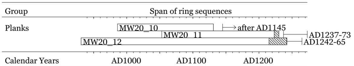
Figure 6: Bar diagram of dated plank samples, indicative felling dates based on an Irish sapwood estimate of 14–50 years. Sapwood is shaded
