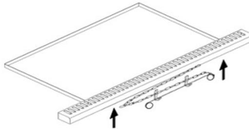
**INFRARED “BACK BURNER”** The rear Infrared Back Burner allows for slow rotisserie cooking of meats and poultry. Infrared burners radiate heat onto the outer surface of the food. This allows cooking without the grease drippings burning on the flame tamers.
