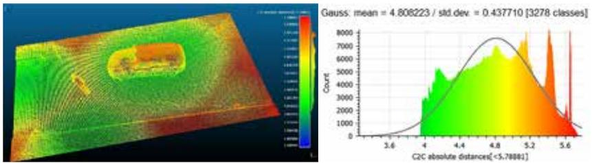
**FIGURE 10:** An accuracy assessment of a 45 mm focal length RGB camera point cloud (data product-4, geo-referenced using the drone's onboard GNSS), against terrestrial scanner benchmark data in the three-dimensional direction ( $x$ ,  $y$ , and  $z$ ).
