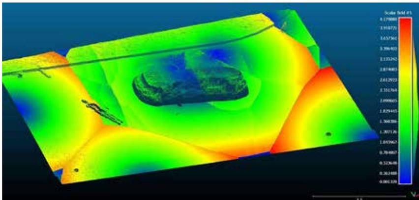
**FIGURE 11:** An accuracy assessment of a 45 mm focal length RGB camera point cloud (data product-4, geo-referenced using the drone's onboard GNSS), against terrestrial scanner benchmark data in the two-dimensional direction ( $x$  and  $y$ ).
