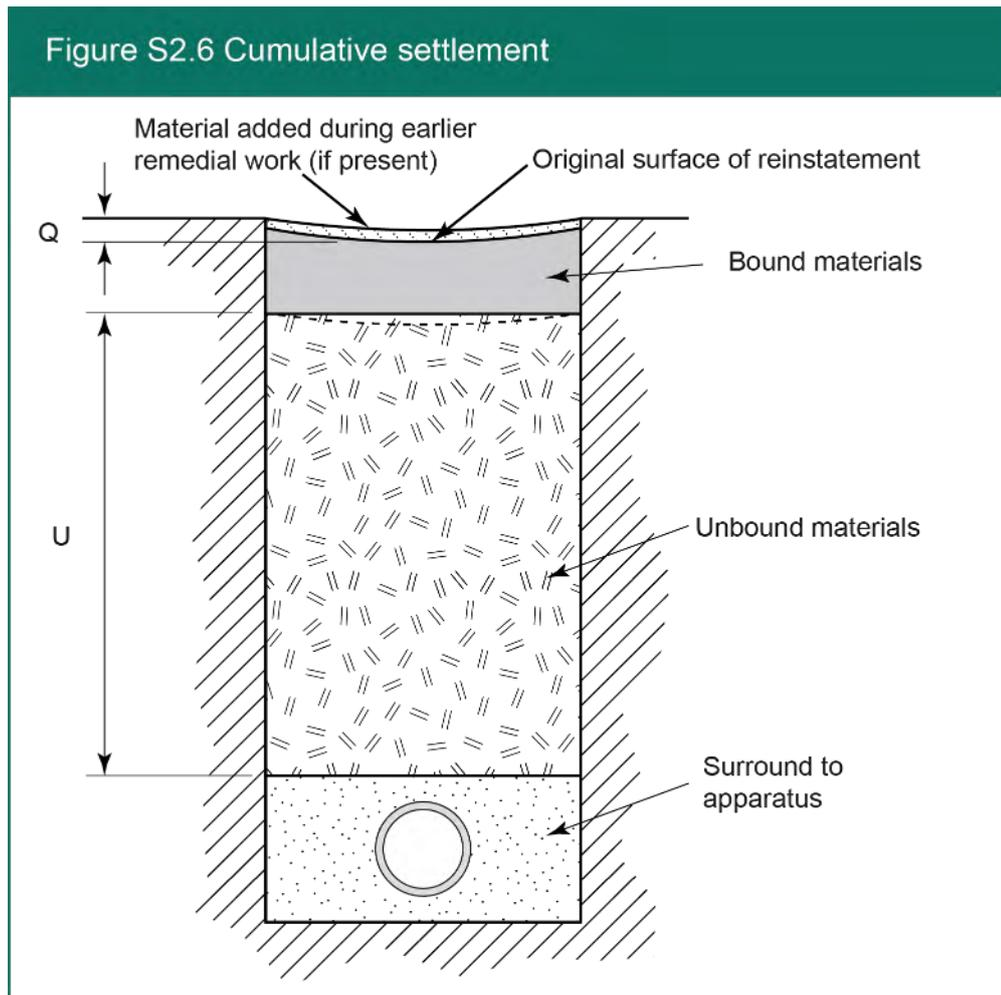
**S2.5.2** If the cumulative settlement of a reinstatement exceeds the limits shown in Table S2.4 at any time within the guarantee period, an agreed engineering investigation must be carried out jointly with the authority. The investigation should establish whether settlement is likely to continue and determine the extent of remedial action required.
