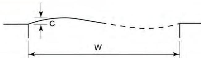
C is the Surface crowning contribution. If this value is greater than the combined defect intervention limit specified in Table S2.2, intervention is needed.
