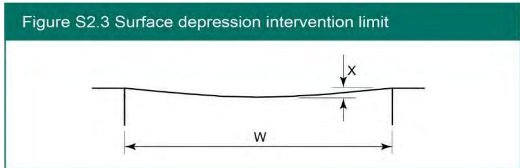
**S2.2.4** Earlier intervention is required if the depression alone results in standing water wider than 500 mm or exceeding 1 m<sup>2</sup> in area, at 2 hours after the cessation of rainfall.
