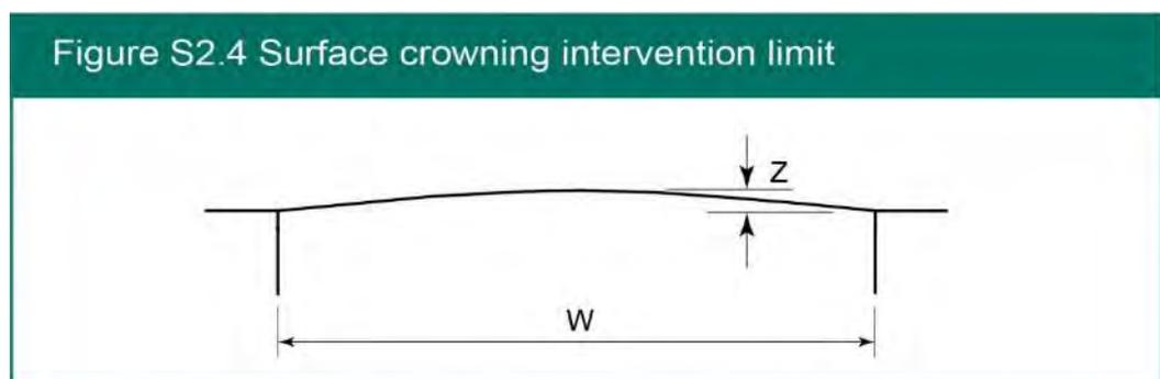
**S2.2.6** Earlier intervention is required if crowning alone results in standing water wider than 500 mm or exceeding 1 m<sup>2</sup> in area, at 2 hours after the cessation of rainfall.
