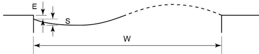
E is the edge depression contribution and S is the surface depression contribution. Once E and S are measured, they are compared with the combined defect intervention limits set in Table S2.1. If E or S is greater than the specified limit, intervention is needed.
