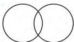
Core re-use is not permitted without the authority's approval when there are more than 2 interlocking large diameter cores (S6.7.4).
