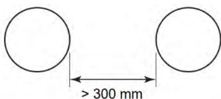
Individual cores are not permitted to be spaced closer than 300 mm without the authority's approval (S6.7.4).
